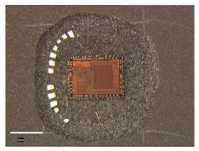
Epoxy package opened with fuming nitric acid (courtesy of C. Toulemont, SERMA)
